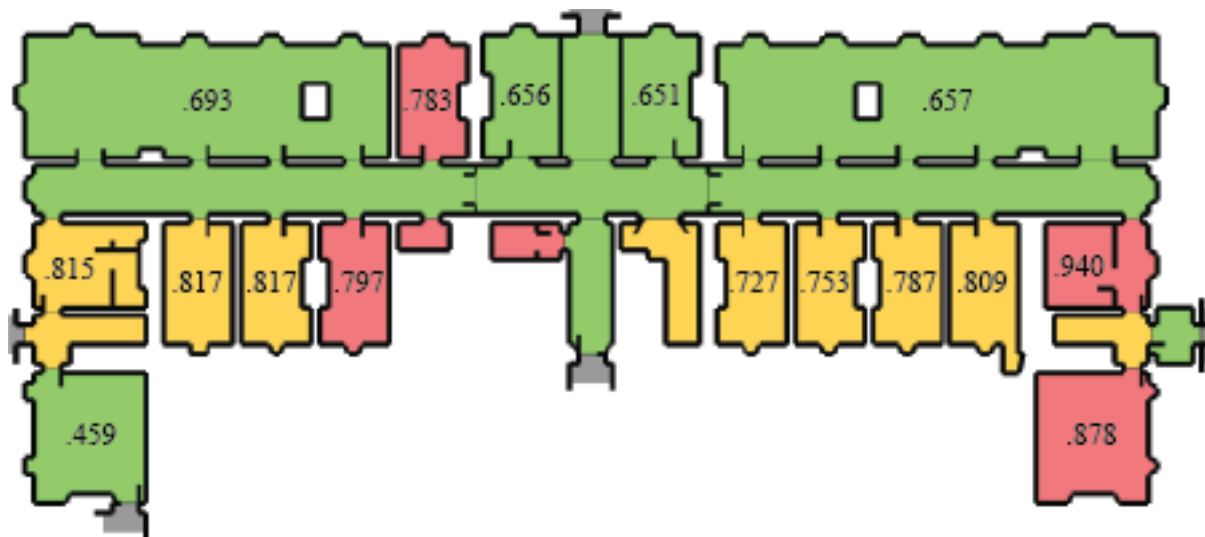
Figure 5: The Rescue Sheet ZONE Colouring of the Geometry with aVEV for Each Room.
