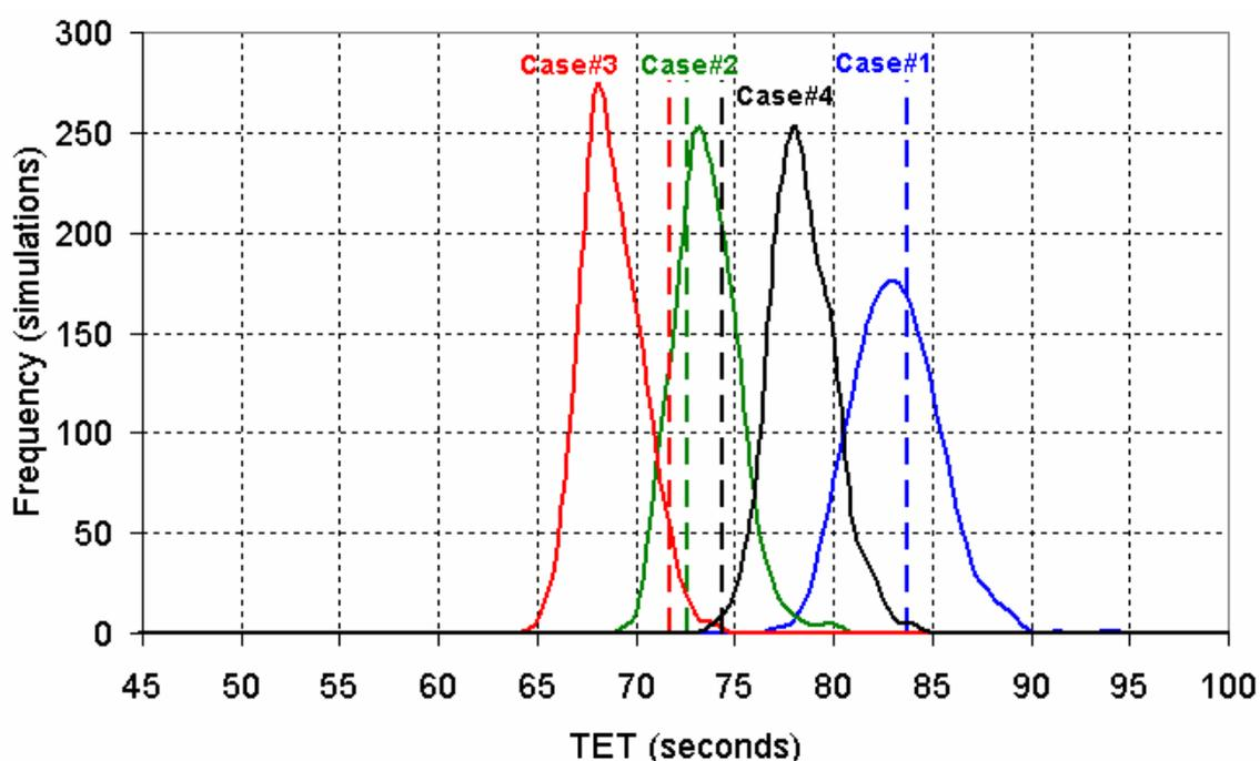
**Figure 12: The frequency distributions of Total Evacuation Times (s) for the four wide body aircraft. (Continuous lines airEXODUS predictions, dashed line represents time achieved in trial).**
