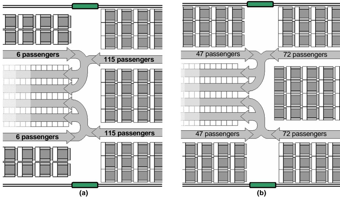
**Figure 32: The number of passenger that would use forward and aft moving passenger aisle for (a) the original design and (b) the alternative design**
