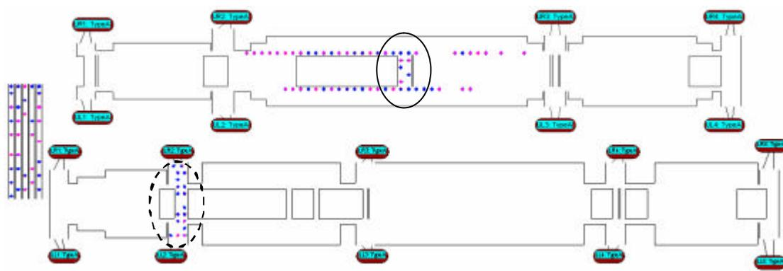
Figure 35: Graphic output from airEXODUS with a 5-lane exit staircase at 46 seconds
