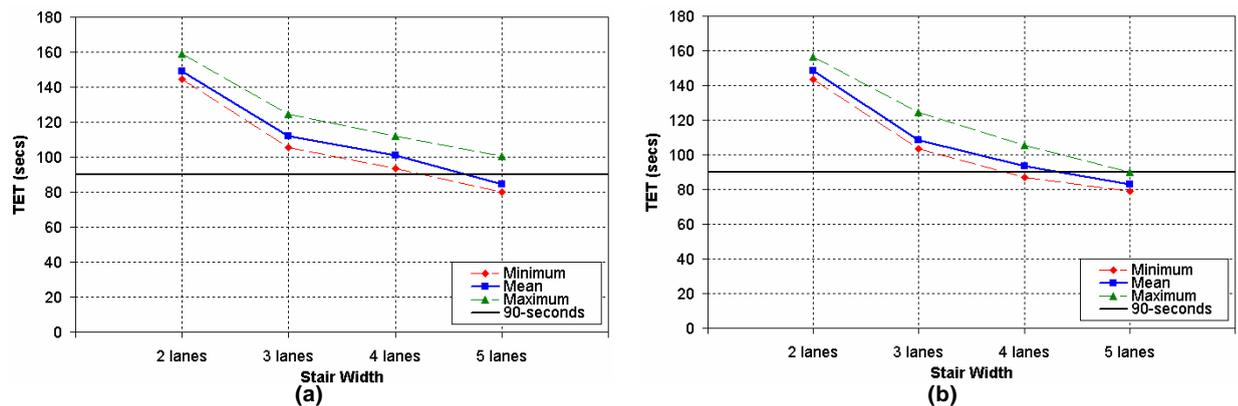
Figure 34: TET as a function of stair lane width for the alternative design (Scenario 3e) (a) without ACCM (b) with intelligent ACCM
