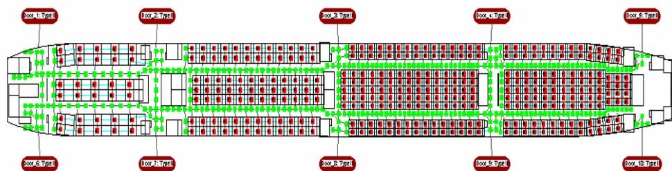
**Figure 6: Cabin layout in airEXODUS. View depicted represents the interactive graphics component within airEXODUS. Aircraft depicted has five pairs of exits. The node structure showing seats, aisles and cross-aisles is clearly depicted.**
