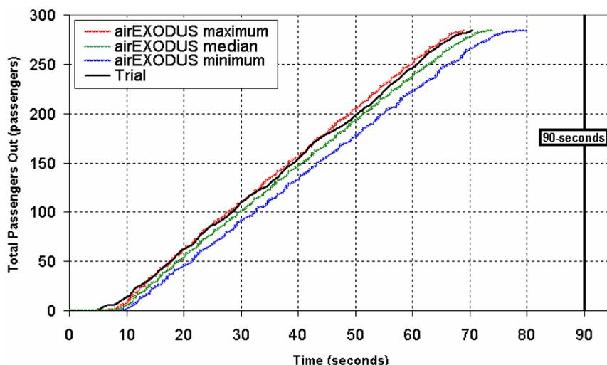
**Figure 13: Cumulative exit times for CASE 2 trial result (Black) and predictive envelope created from airEXODUS simulations.**
