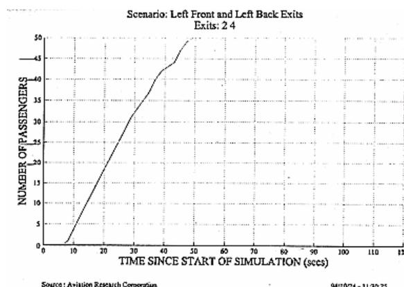
Figure 4: Example output from the ARCEVAC model
