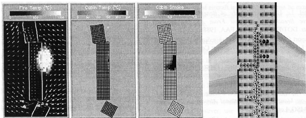
**Figure 9: Screen shot of the output from Macey's model. Left is the airflow model, centre is the thermo-toxic model, and right is the evacuation model**
