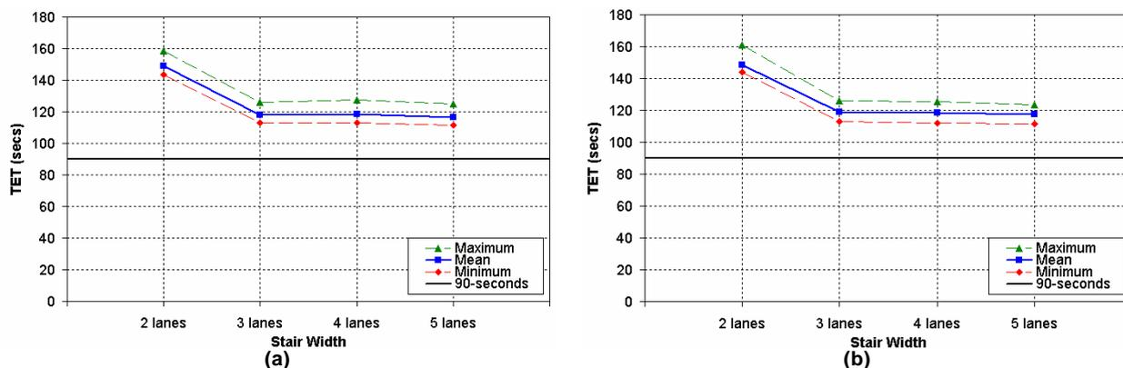
**Figure 29: TET as a function of stair lane width (Scenario 3d), (a) without ACCM and (b) with intelligent ACCM**
