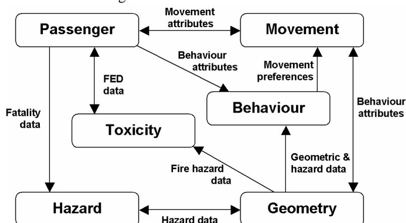
Figure 5: airEXODUS Submodel Interaction
