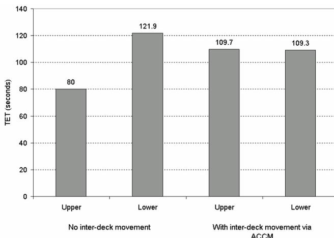
**Figure 37: Summary of the finishing time of upper deck and lower deck exits with and without inter-deck movement**
