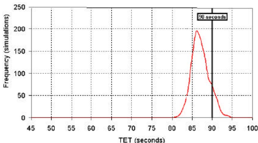
**Figure 15: Numerically generated evacuation time distribution (frequency Vs evacuation time) for a particular scenario for a hypothetical aircraft configuration.**
