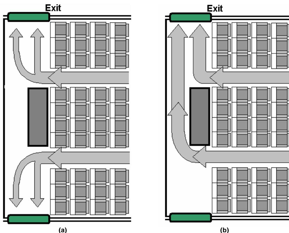
**Figure 21: Hypothetical flow pattern at an end of section exit when (a) both exits from exit pairs are available and (b) one exit from and exit pair is available**
