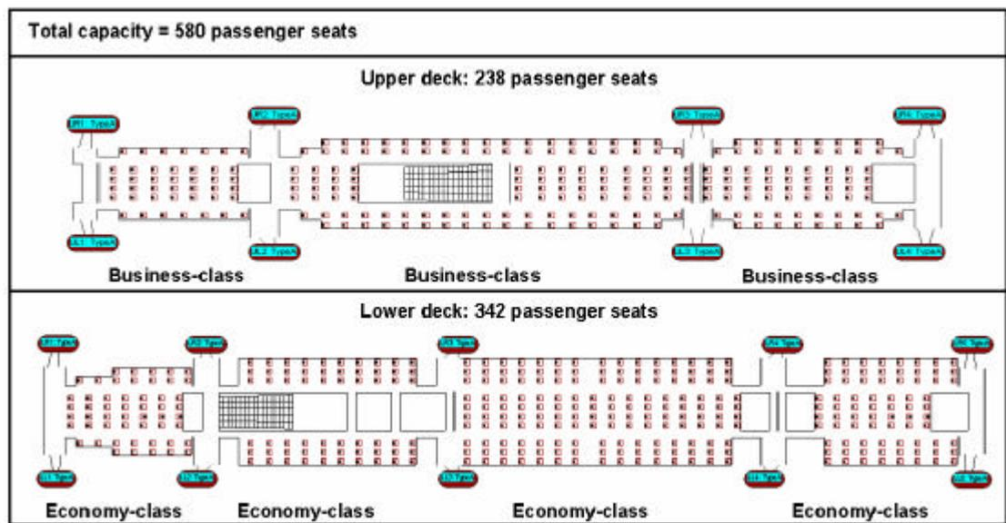
**Figure 31: An alternative design – used in Scenario 3e - in which the top of the staircase is centrally located within the upper deck**
