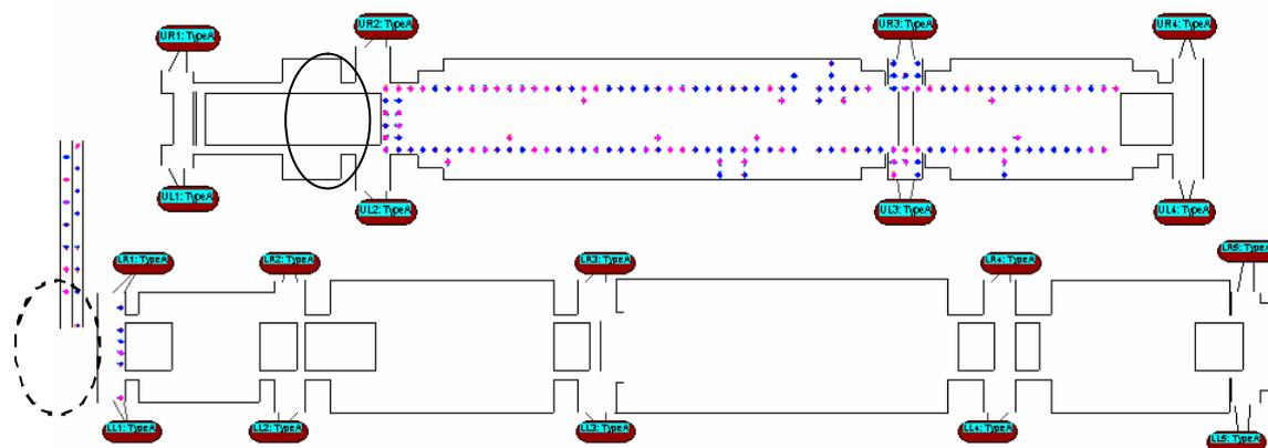
**Figure 25: Graphic output from airEXODUS showing congestion at the top of the stairs 48 seconds after the start of the evacuation**
