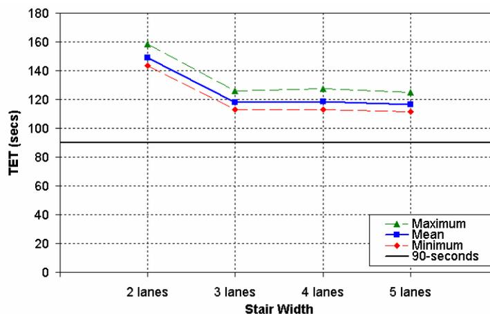
**Figure 28: TET as a function of stair lane width**
