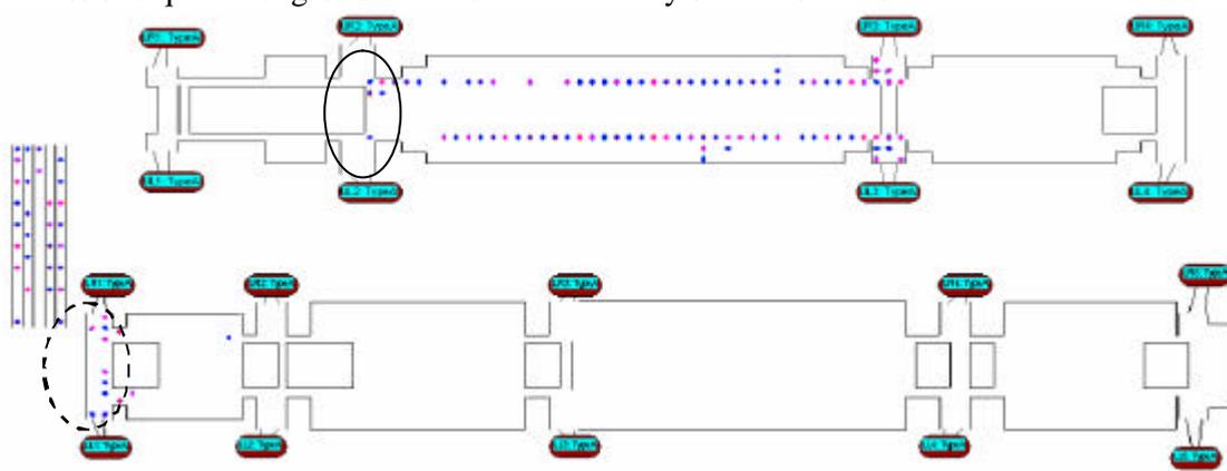
**Figure 30: Graphic output from airEXODUS with a 2-lane exit staircase at 55 seconds when Active Cabin Crew Management**
