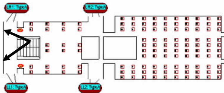
**Figure 26: The cabin crewmember redirection stations (denoted by arrows) on the lower deck**
