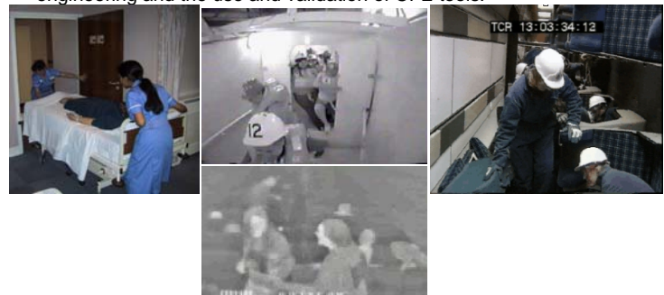
Evacuation Trials: FSEG conduct evacuation trials in a range of environments including hospitals, ships, rail carriages and smoke filled aircraft cabins in order to collect human performance data
