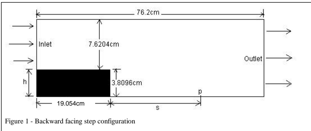
Figure 1 - Backward facing step configuration
