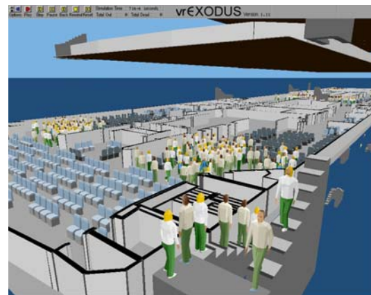
Figure 3: vrEXODUS output showing mustering in a large passenger ship.
