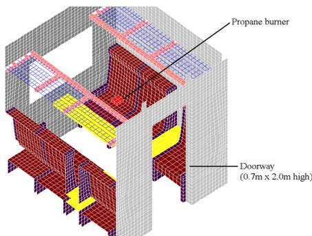
Figure 2 Setup with mesh size of around 0.06 m
