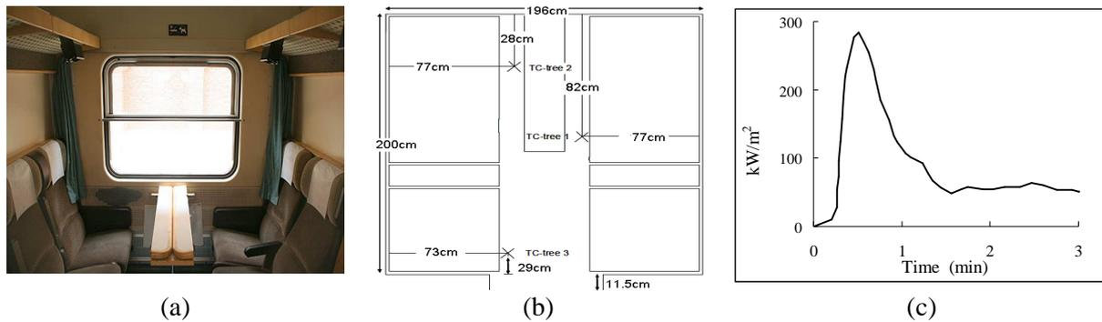
Figure 1. (a) Interior and (b) top view of the compartment; (c) Cone calorimeter HRR data for seats
