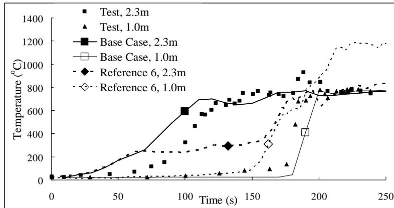
Figure 5 Measured and predicted temperatures at thermocouple tree 3.
